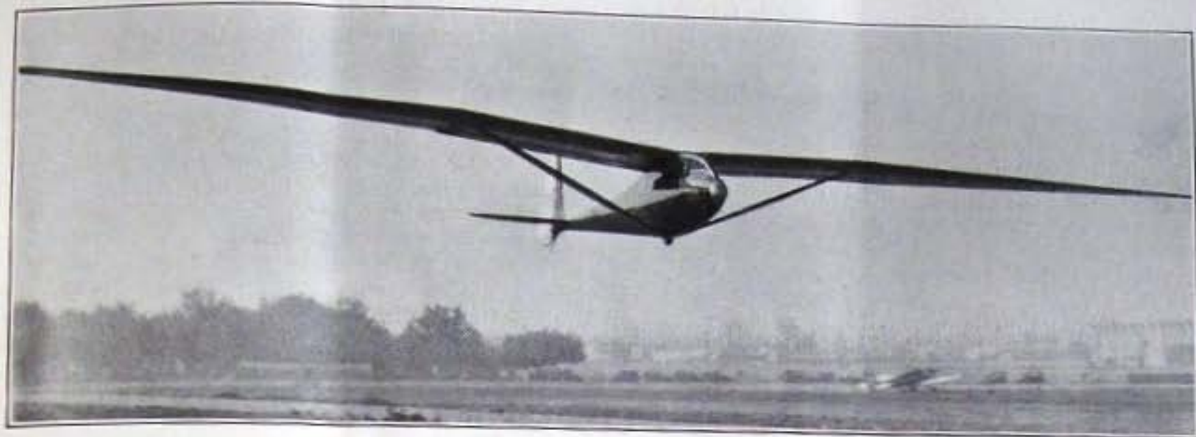
The "Albatross I," named "Falcon," which has a mahogany plywood skin. It was built for the late Warren Eaton.
